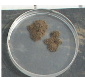
Slaking Soil (Poor Quality)
