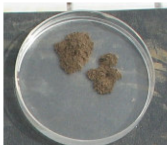
Slaking Soil * (Poor Quality)
