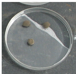
Non-Dispersive & Non-Slaking Soil (High quality)
