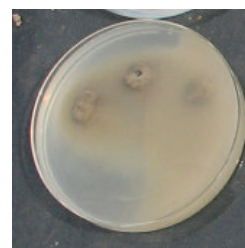
Dispersive Soil (Poor Quality)
