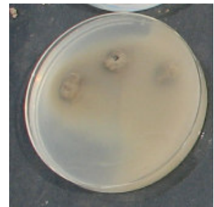
Dispersive Soil (Poor Quality)
